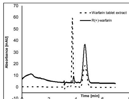
**Figure 4.** Chiral HPLC separation of warfarin tablet extract (---) and standard R(+)-warfarin (—)
