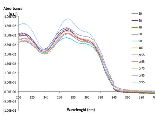
**Figure 2.** UV - reflectance spectra of training and validation set of varying mole fractions of R-(+)-warfarin in the presence of 3.24mM tert-butyl-calix[6]arene; 200-400 nm
